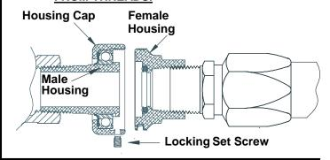
**Step 5:** Remove the Seal and O-Ring from the Female Housing.
