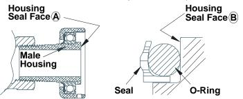
**Step 7:** Lightly lubricate the replacement O-Ring only with Dow 111 lubricant (provided when Seal Kit is ordered).
